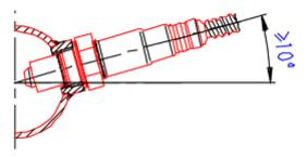
• For hot applications (temperature of hexagon above 500°C \*) the thread boss should be at least 13 mm or longer to avoid overheating of the protection tube welding and to cool down the sensor hexagon.
