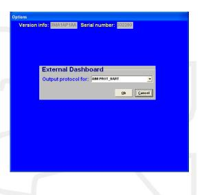
For the new AIM displays with new firmware you can select the KMS protocol in the AIM software. In the KMS software please select AIM\_KMS for this protocol. Even more options are available with this communication protocol. The channels that can be transmitted to the AIM display are shown in Appendix 2: AIM display connection and channels. Please contact your AIM dealer for more details.
