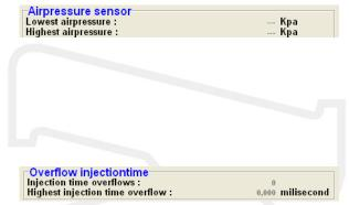
For example a injection time of 23 ms and a engine speed of 6000 rpm. The time of 2 rotations =  $1/(rpm/minute)x^2 = 1/(6000/60)x^2 = 20 ms$ . The overflow is 23 - 20 = 3 ms. When choosing injectors it's important that the flow is high enough so that injection time doesn't
