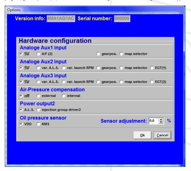
Here the different functions for each analog input can be defined, depending on the way the different functions are connected/wired. The connection/wiring of the analog inputs for different functions are shown in the wiring diagrams on the following pages.
