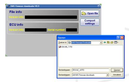
For IA23 the update file name starts with the number 2 and has extension \*.FIO. It's only possible to use this firmware downloader if you have an KMS ECU with serial nr. higher then 300000.
